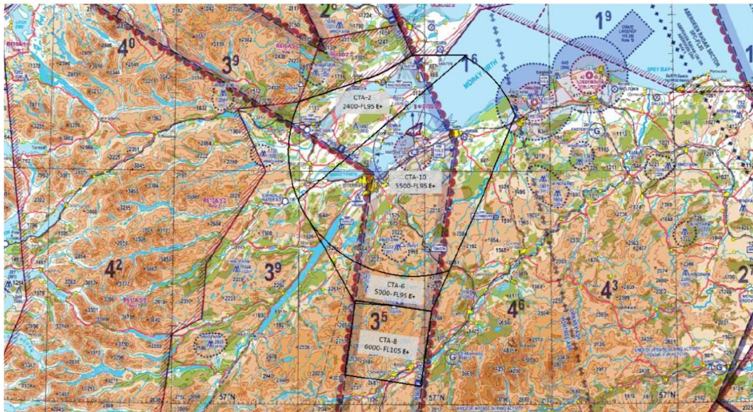
Figure 4 Geographic extent of the Inverness Control Zone (CTR) and Control Areas (CTA) UK Civil Aviation Authority (CAA) / NATS Digital Data. VFR Chart Scotland, 500,000, June 2013
